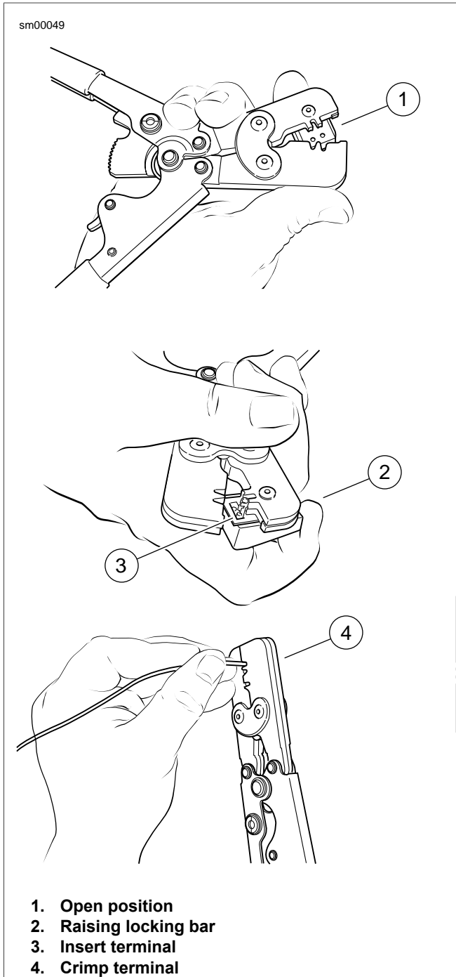
Figure A-27. Delphi Micro-64 Sealed Connector: Terminal in Crimper
